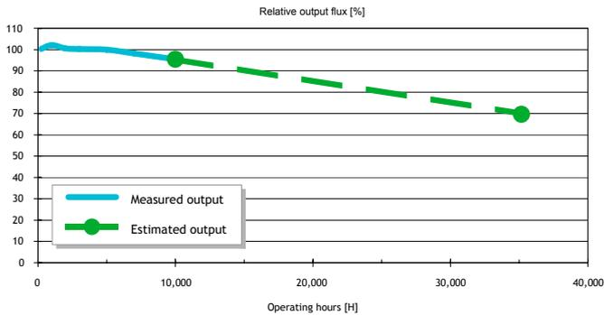
Expected output depreciation at 45°C ambient. Plots are based on the LED manufacturer's ongoing end-of-life tests after 10,000 hours. The 35,000-hour lifetime (L70) is accepted in accordance with IESNA LM 80-08 if the lumen maintenance is minimum 94.1% after 6,000 hours of operation. The LED manufacturer's measurements show that the actual level is minimum 98.5%.
