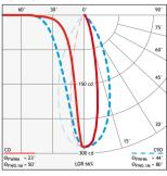
$\Theta_{\text{FWHM}}$  is the full-width beam angle where intensity is half the maximum level.  $\Theta_{\text{FW0.1M}}$  is the full-width beam angle where intensity is a tenth of the maximum level. This is a non-standard measurement that is close to the perceived beam angle.
