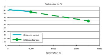
Expected output depreciation at  $45\,^{\circ}\text{C}$  ambient. Plots are based on the LED manufacturer's ongoing end-of-life tests after 10,000 hours. The 35,000-hour lifetime (L70) is accepted in accordance with IESNA LM 80-08 if the lumen maintenance is minimum 94.1% after 6,000 hours of operation. The LED manufacturer's measurements show that the actual level is minimum 98.5%.
