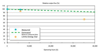
Expected output depreciation at  $45^{\circ}$ C ambient/ $105^{\circ}$ C junction at 1000mA lf. Measurements are based on the LED manufacturer's IESNA LM80-08 tests. The 6,000 and 35,000-hour lifetime (L70) limits are accepted in accordance with IESNA LM 80-08. The estimated data is calculated using the same methodology. The LED manufacturer's measurements show that the actual level after 6,000 hours is 98.7%.
