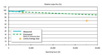
Expected output depreciation at  $60^{\circ}\text{C}$  ambient/145 $^{\circ}\text{C}$  junction at 600mA If. Measurements are based on the LED manufacturer's IESNA LM80-08 tests. The 6,000 and 35,000-hour lifetime (L70) limits are accepted in accordance with IESNA LM 80-08. The estimated data is calculated using the same methodology. The LED manufacturer's measurements show that the actual level after 7,000 hours is 98.7%.
