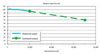
Expected output depreciation at  $45\,^{\circ}$ C ambient. Plots are based on the LED manufacturer's ongoing end-of-life tests after 10,000 hours. The 35,000-hour lifetime (L70) is accepted in accordance with IESNA LM 80-08 if the lumen maintenance is minimum 94.1% after 6,000 hours of operation. The LED manufacturer's measurements show that the actual level is minimum 98.5%.
