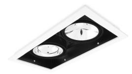
Resourceful, discreet multipurpose LED downlight. Recessed. Low-glare. Each head tilts 30° in all directions. For indoor use. For area, room, display, surface and task lighting. Easy installation in any ceiling. Xicato LED technology. Choice of CCT, lumen and beam angle combinations. Minimum 50% energy saving compared to equivalent halogen. Light quality ensured for entire lifetime. Rigorously tested. Rigorously documented. The light you specify is the light you get.
